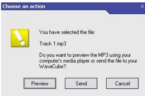
Once you have located an MP3 file, a single mouse click will display the full filename and file size at the bottom of the WaveCube window. The maximum size file you can send to the WaveCube is 12 megabytes (12,000 KB). Double-clicking on an MP3 file will bring up a prompt window. (Illustration 1.8)
